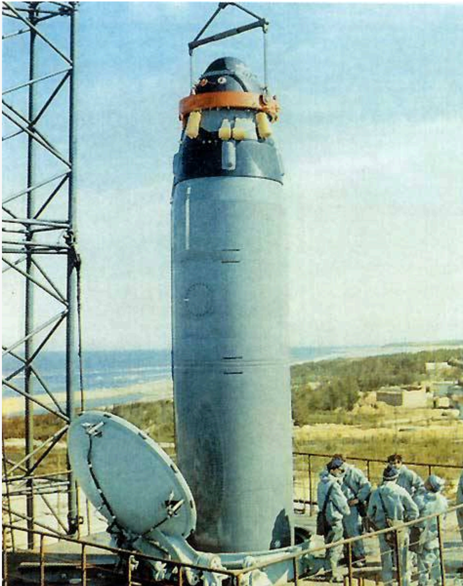
Loading an experimental rocket into a launcher at a land test site. Photo Rbase.new-factoria.ru
